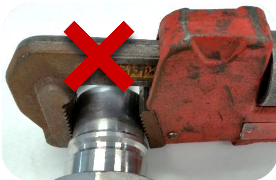
Figure 15 - Improper Use of Hand Tool
