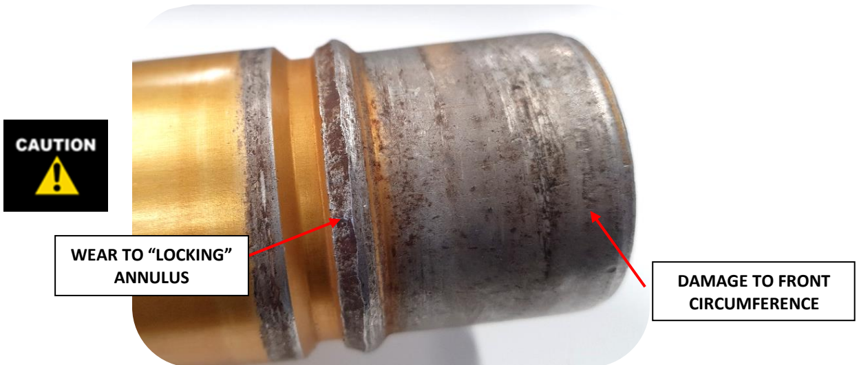
Figure 19 – Excessive Wear to Ball Lock Annulus
