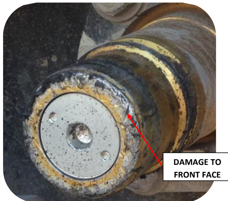
Figure 20 - Wear to Front of a non-Banlaw Aluminium Receiver
