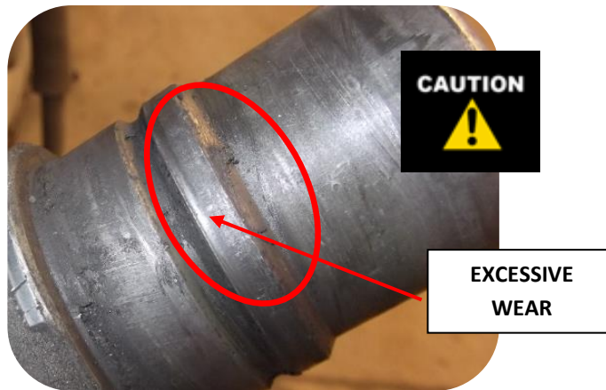
Figure 21 – Excessive Wear to Ball Lock Annulus
