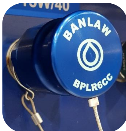
Figure 10 - Receiver Dust Cap Fitted
