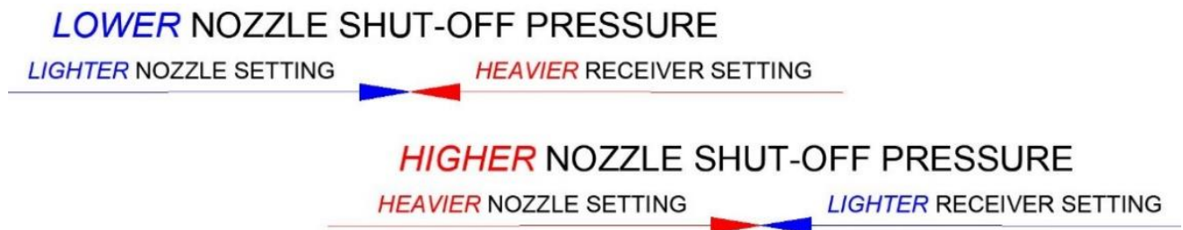
Figure 10 - Relationship Between Nozzle and Receiver Spring Settings
