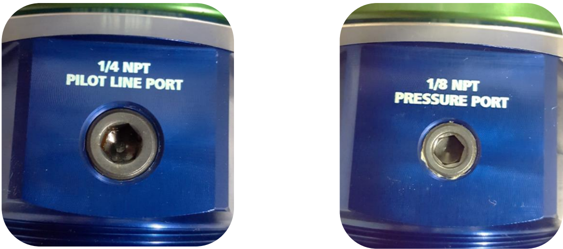
Figure 2 - External Pilot Line and Tank Pressure Indicator Ports (normally plugged/sealed)
