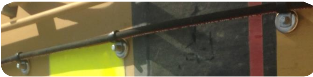
Figure 10 - Example of External Pilot Line Retention
