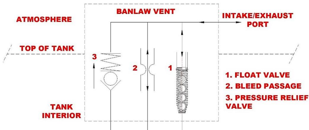
Figure 3 - Generic Process Flow Paths for Banlaw Vent
