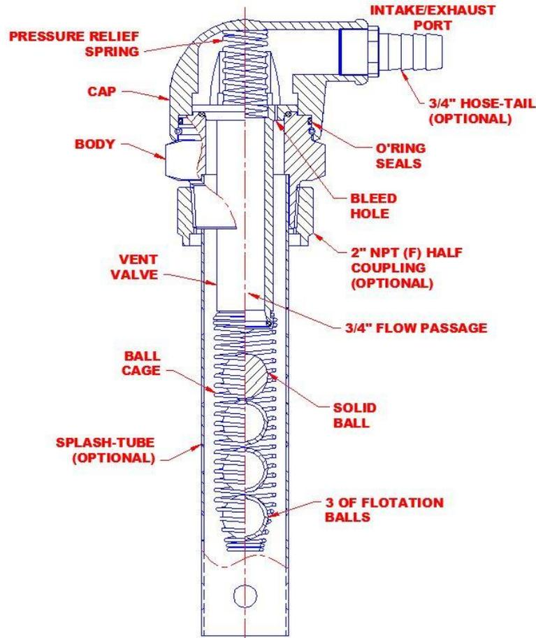
Figure 2 - Partial Section View of Vent with Generic Features
