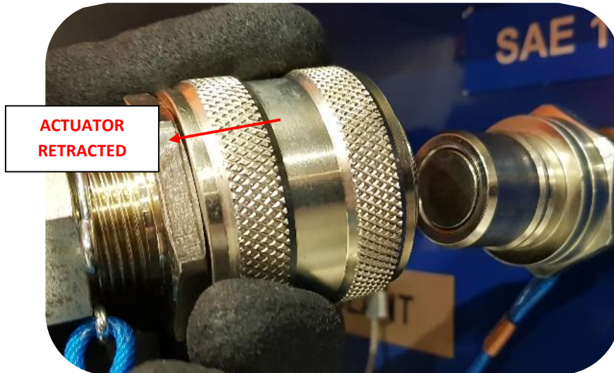
Figure 7 - Nozzle Actuator Retracted prior to Connection
