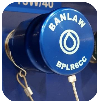
Figure 9 - Receiver Dust Cap Fitted
