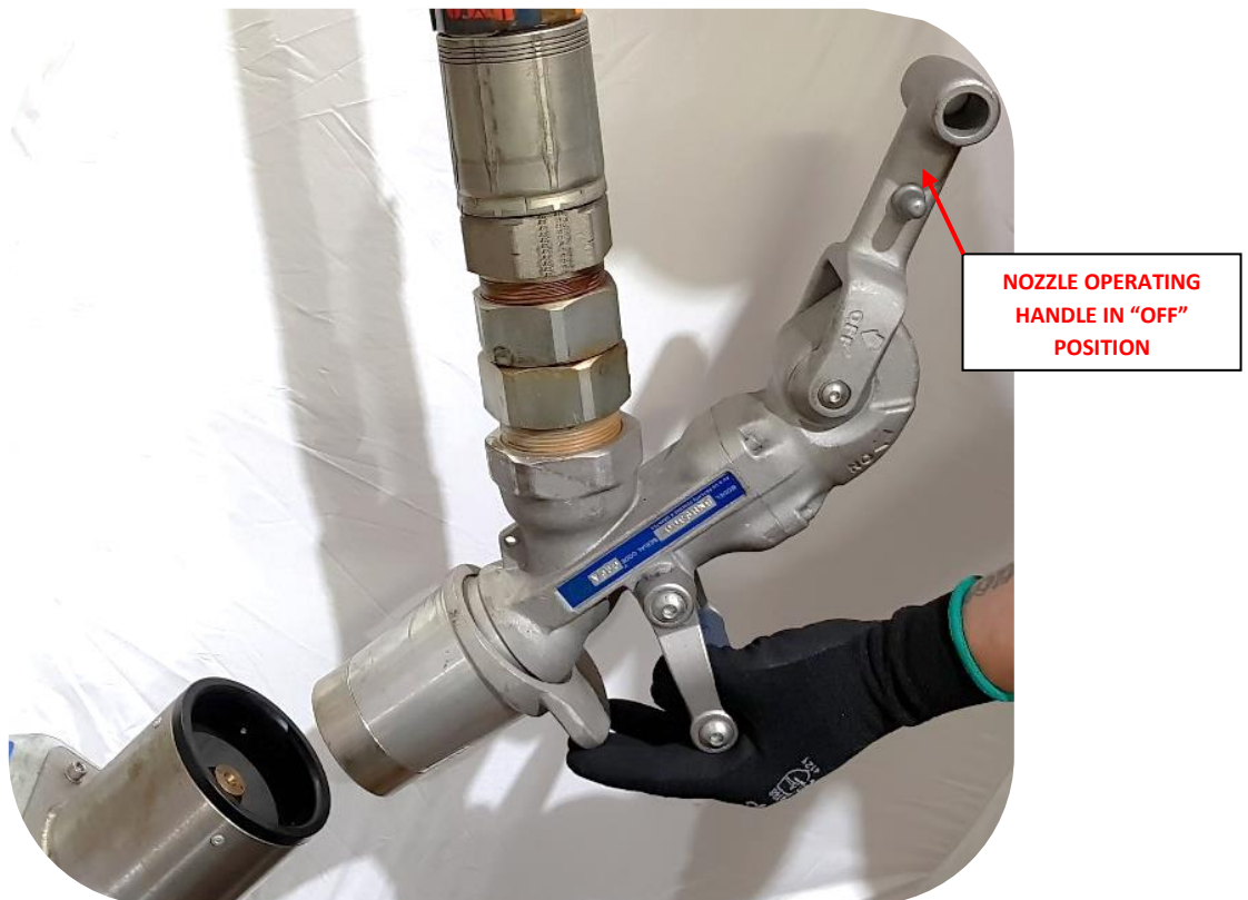
Figure 7 - Preparing the Nozzle for Placement into the Holster
