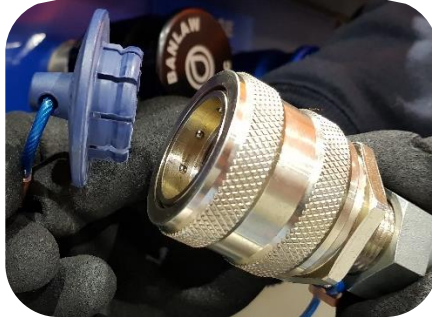
Figure 5 - Dust Plug removed from a Nozzle
