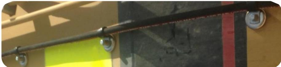
Figure 11 - Example of External Pilot Line Retention
