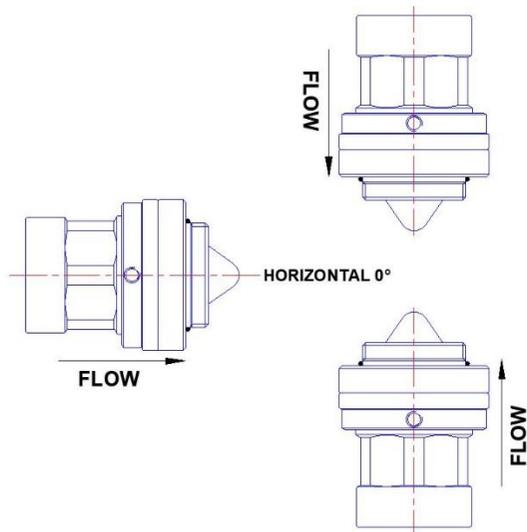
**Figure 10 - Angular Limits of Valve Operation**
