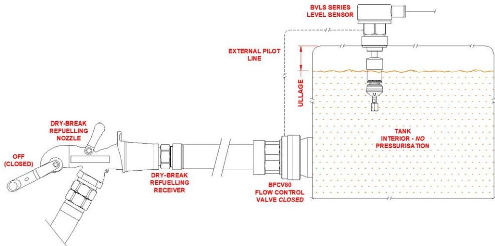
Figure 9 - Tank Filled
