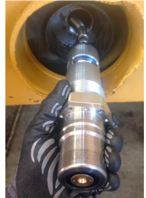
Flow Control Valve with integrated Auto ID receiver being installed
