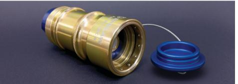
The BEC-B does not include the manual open/close valve found in our BEC. Because of this, there is no requirement to 'twist' the BEC-B to unlock the fluid path. It is designed for tighter service boxes, where there isn't room for a tool as well as a pair of hands.
