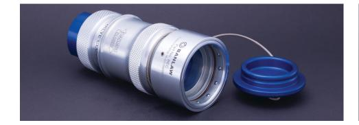
The BEC has a fluid-tight connection, which prevents spillage during the evacuation process. It is Dry Break and incorporates a dependable ball-lock latching mechanism. As with the entire LubeCentral range, the BEC fluid path is optimised for higher transfer rates.
