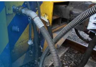
Banlaw has used its design expertise to solve the problem of **Pacific National operators** being doused in fuel when disconnecting in-line refuelling hoses between tanks and locomotives.
