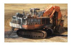
This picture was taken after a fuel fed fire at an Australian mine that put the driver in hospital, wrote off an expensive excavator and caused significant lost production.
